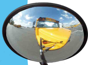
Rosco Hawk-Eye® cross view mirror without partial tint
